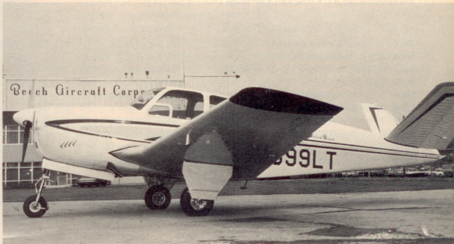
FIGURE 4 Here, in rear cg condition, Bonanza shows weight thrown on main struts, nose gear strut is fully extended
